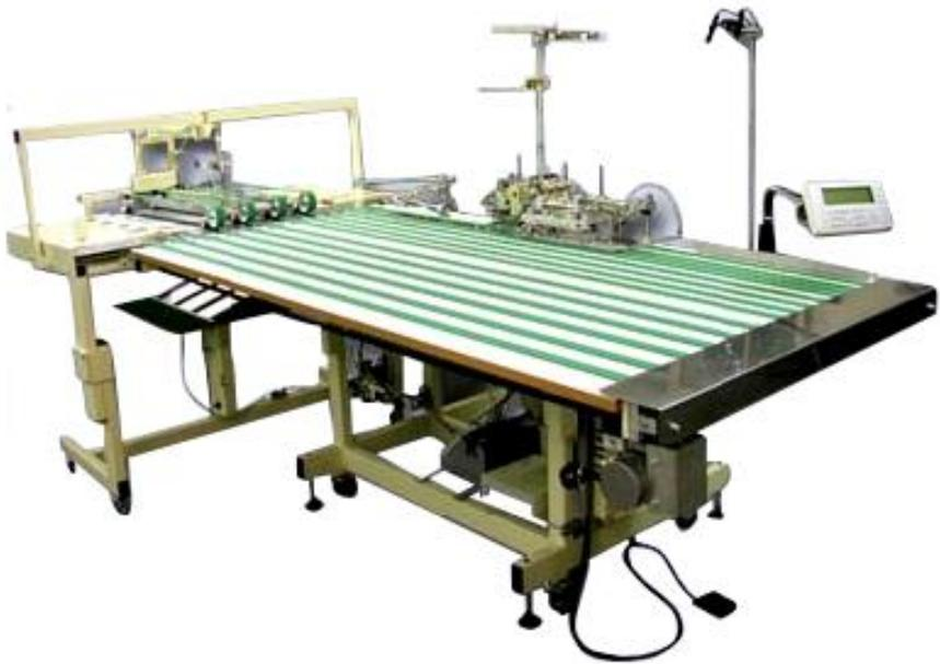
lockstitch Sahl Workstation, with a Re-entry system to attach either flat or folded tape; the tape is automatically cut and ensures that the tape or collar is never twisted. (Less rejects)
